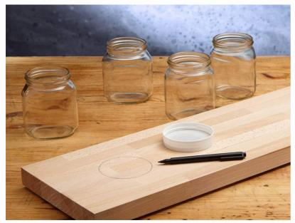
Using the lid as a template: use a pen to draw an outline around the lid, so you can gauge the distance accurately and see exactly where the lids have to be screwed on.
