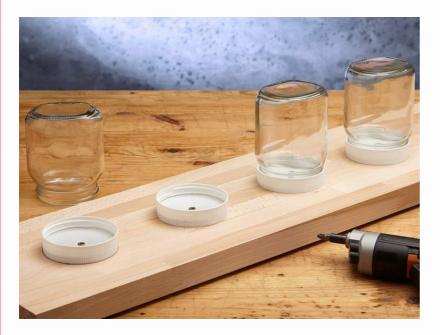
Now position the lids on the points you have marked, and drive a screw through the middle of each one.
